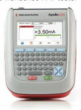
A straightforward electrical safety tester with QWERTY keypad for fast data entry and storage of up to 2,000 appliance records.
