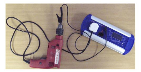
Press the Class II button. The MemoryPAT will first check that the power switch on the item is in the ON position. If it is then the testing will begin. If the user has forgotten to switch the appliance ON then the MemoryPAT will display the following reminder message.
