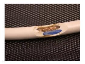
Damage to power cable sheath.
