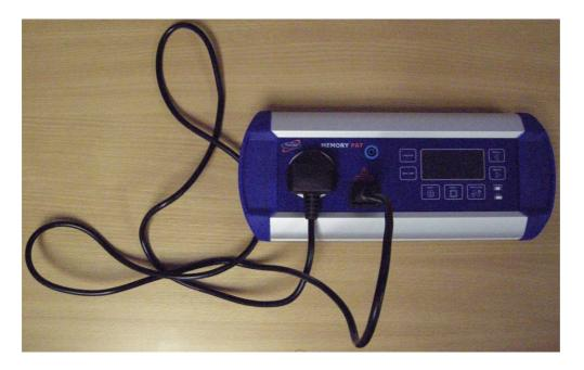
For IEC leads up to 1 metre in length, press the Power cord button. The MemoryPAT run through the tests and the results for Insulation Resistance, Earth Continuity, and Wiring will be displayed as well an overall Pass or Fail as shown below.
