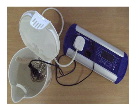
Press the Class I button. The MemoryPAT will first check that the power switch on the item is in the ON position.
