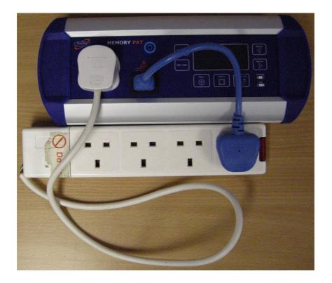
For mains extension leads up to 1 metre in length press the Power cord button. The MemoryPAT will run through the tests and the results for Earth Continuity, Insulation Resistance and Polarity will be displayed as well an overall Pass or Fail as shown below.
