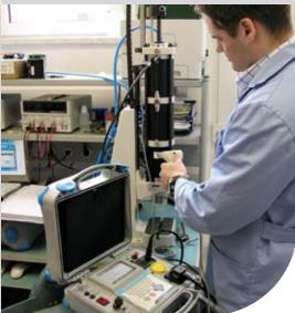
Metrel's top of the range measuring instrument for electrical safety testing of a wide range of (portable) electrical appliances, IT equipment, IEC cords and portable RCDs with corresponding IEC/EN and VDE standards.
