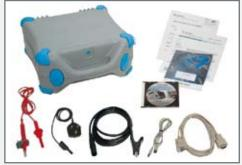
Instrument OmegaPATPlus MI 3305 or BetaPATPlus MI 3304 Earth Bond Clip PRCD test probe Flash Test Probe (only for MI 3305) PC SW PAT Link with RS232 and USB cable Instruction manual Product verification data
