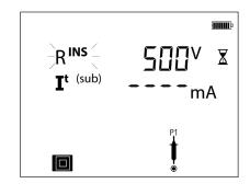
Repeat contact on all exposed conductive parts
