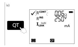
Example 2 – Class II 250 V Insulation test
