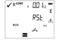
Press TEST button on RCD
