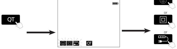
Connection for individual tests differs depending on the test group selected.
