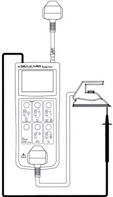
Figure 5. Testing CLI appliances, mains leakage
