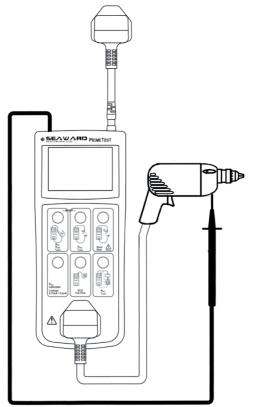
Figure 6. Testing CLII appliances, mains leakage
