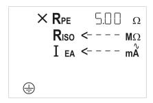
If the measured value is less than the factory set pass/fail threshold, the measured value is displayed and the unit indicates a pass result, as shown below.
