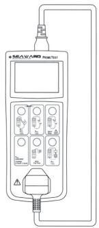
Figure 7. Testing IEC Leads
